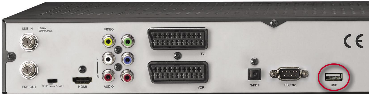
■ USB host interface of the TF7700HSCI for connecting external storage media
