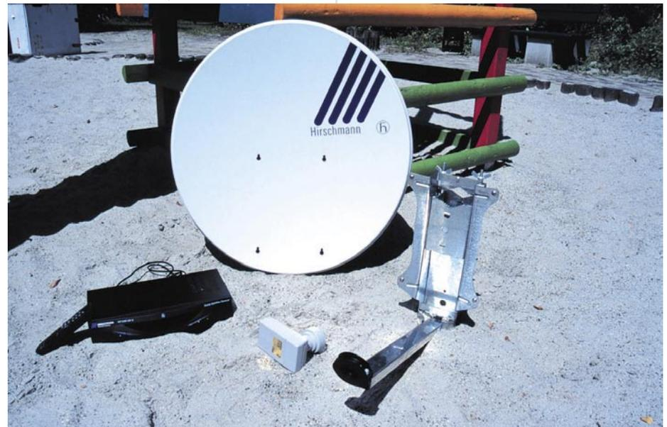
The included LNB is a Twin LNB, so it is very easy to connect an additional digital receiver, which can be operated completely independent of the analogue box. Another fine solution could be the use of one dish for two households.
