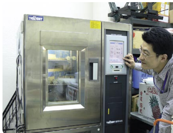
Samples are taken off of the production line and tested in combined hot/cold environmental chambers. Here the oven is heated to 70°C. Tests are conducted from -40° to +90°C.
