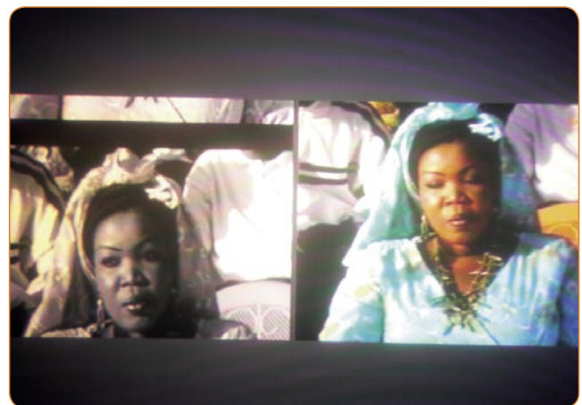
Tony can test two receivers by splitting the video inputs of his Sony TV. In this example he shows us a PAL signal from the Quali HD receiver in the image to the left. The image to the right shows the same channel from a Fortec Star receiver using an LNB splitter. This allows him to confirm whether or not PAL signals are correctly converted into NTSC.
