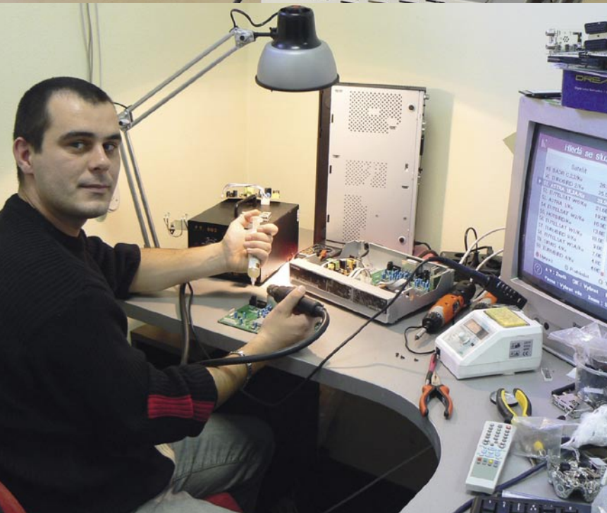
■ Even a top-quality product may fail at some point. Peter Ciljak is one of ABC BIZNIS two technicians. Here he is seen replacing a faulty chipset on a motherboard.
