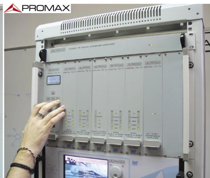
■ The theory is demonstrated via an actual connection: each slot represents a possible signal source. At the other end you get a combined signal in DVB-T.
