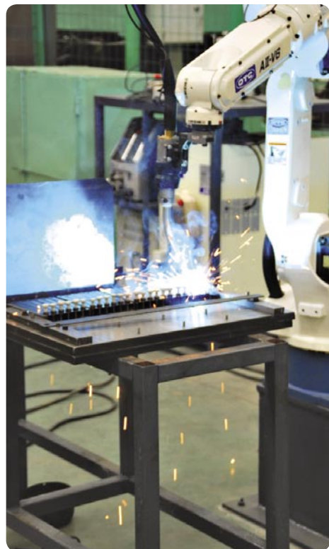
■ Automatic welding robots are used in the production of the support rods.
