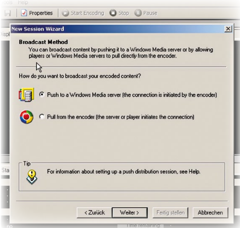
■ Either a direct connection is created or the stream is sent to a server
