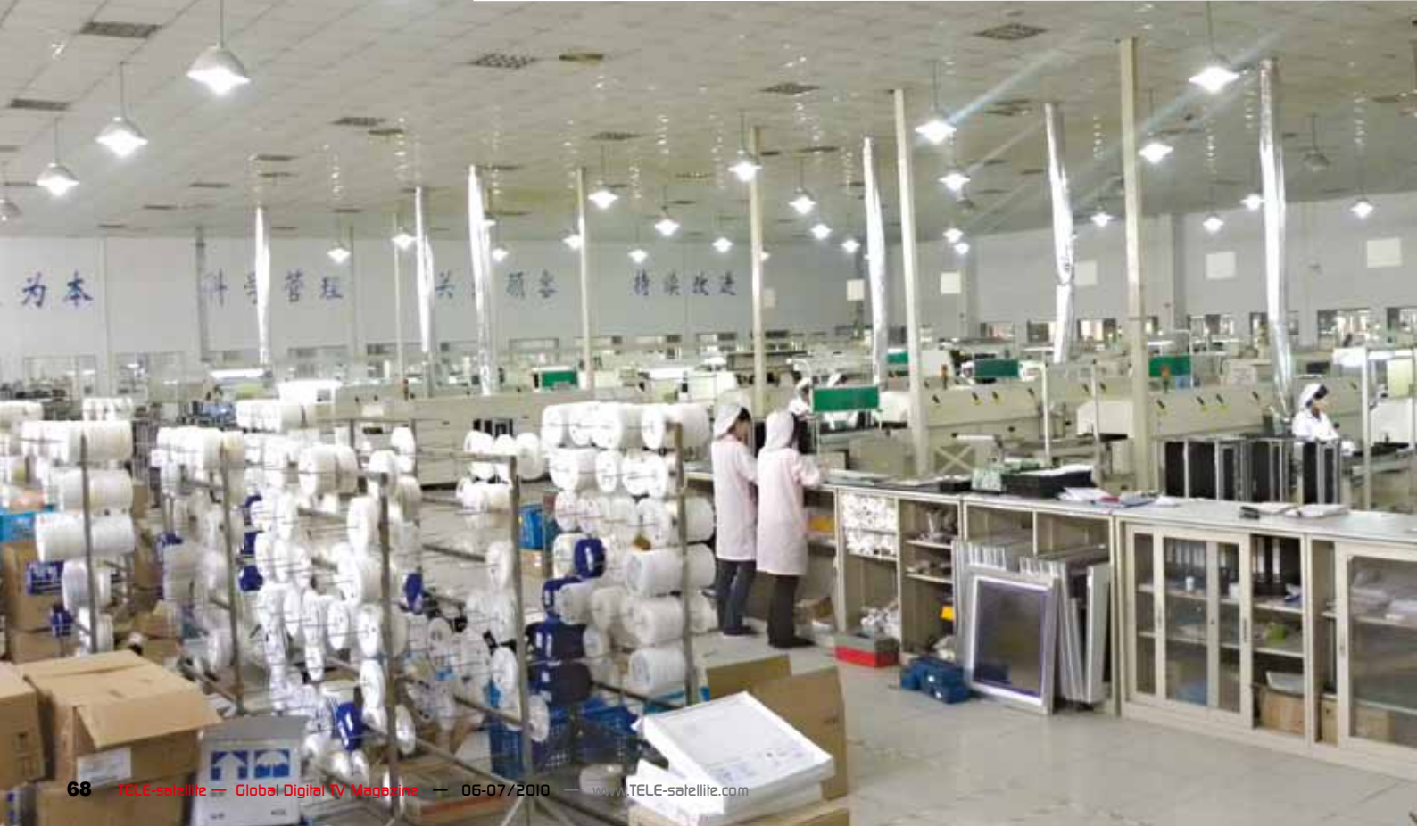
■ At the other end are the rolls with the surface mount components. They are continuously fed by an employee into the SMT automatic mounting machines. The SMT automatic machines run 24 hours a day. The Chinese writing on the wall in the background reads: "Work with Your Fellow Employees; Good Management; Customer Orientation; Continuous Improvement".
