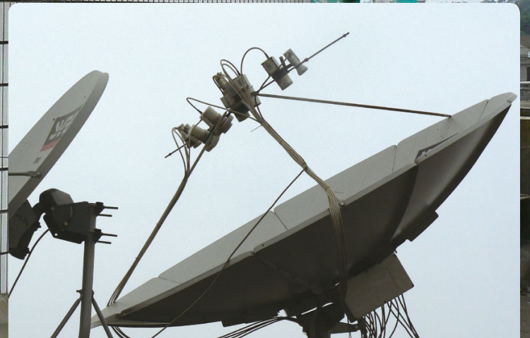
■ Using an extension rail Pepsi has converted his 2.4 m antenna into a multi-feed dish for reception of nine different satellites.
