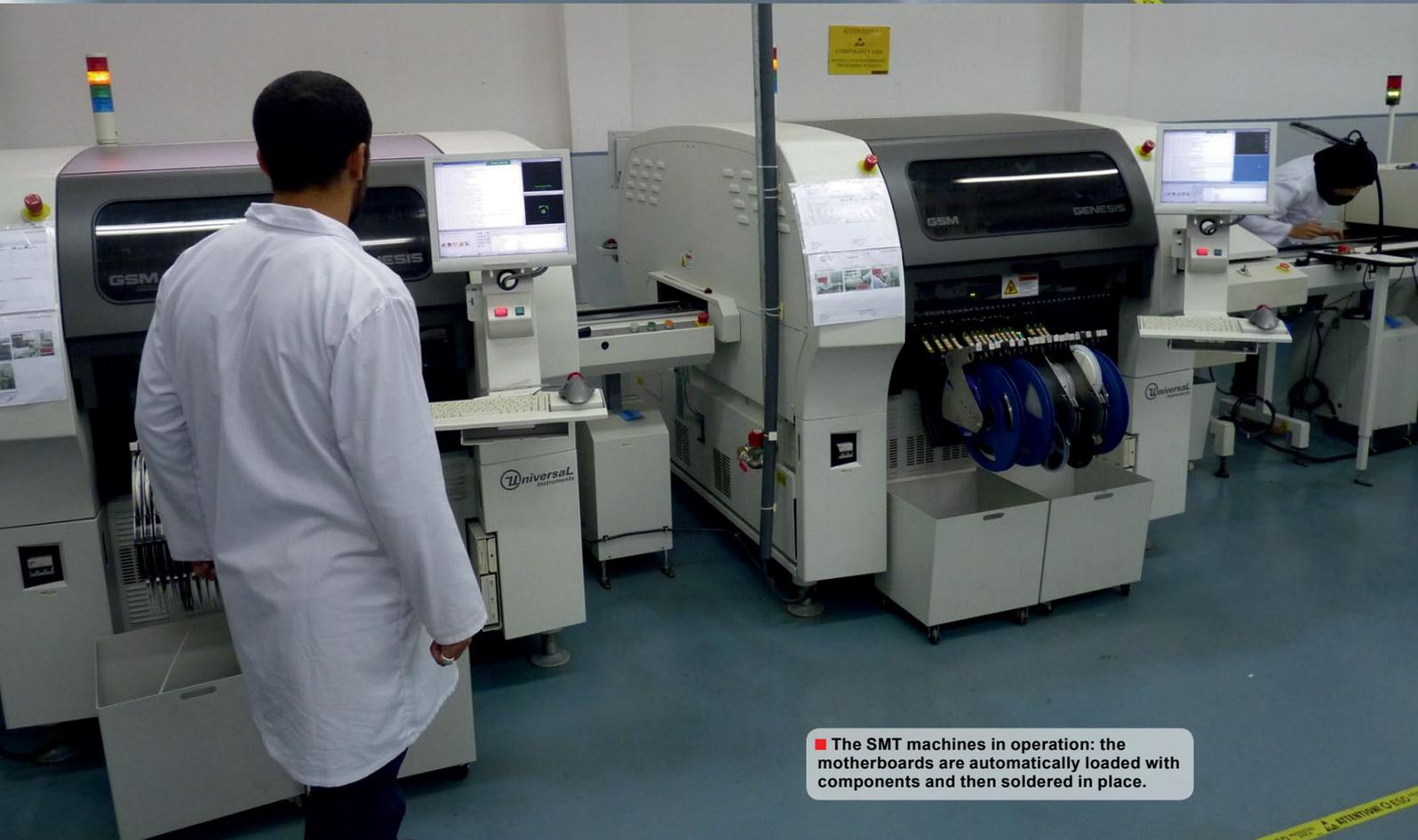
■ The SMT machines in operation: the motherboards are automatically loaded with components and then soldered in place.
