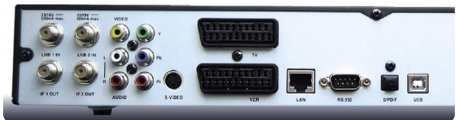
Topfield's TF6000PVRE has a Ethernet connector and can be controlled via a web interface from remote
