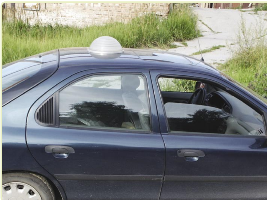
Application of a 3D diffractive antenna for satellite TV reception.
