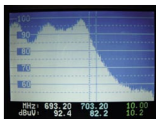
Pengukuran gulungan filter |
