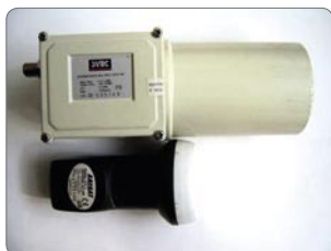
Two regular LNBs – for C-band (top) and Ku-band (bottom)
