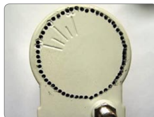
Then we have to drill a lot of small holes around the edge of the C-band's feed rear end
