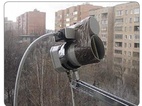
This is how the LNBs are mounted ...
