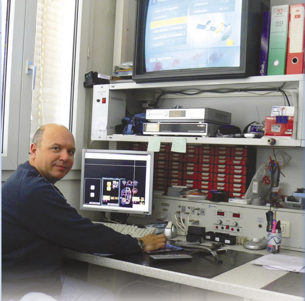
▲ Sandro Gnani is a STAB technician who checks each sample receiver to make sure that USALS has been correctly implemented. The manufacturer can only print the USALS logo on the receiver and its packaging when the receiver has passed every test.
