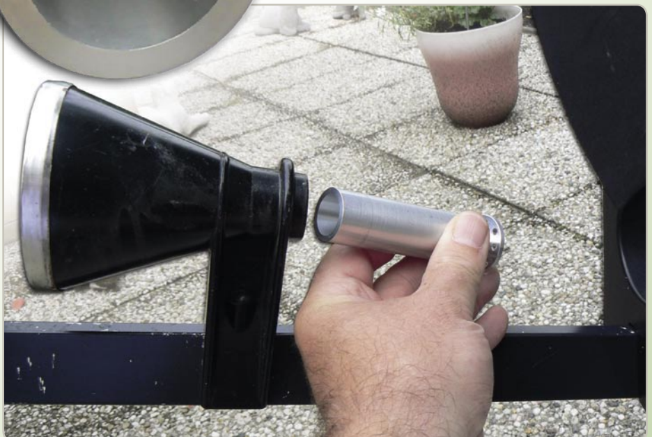
The feed fits perfectly into the existing reflector antenna and is inserted into the existing funnel feed.
