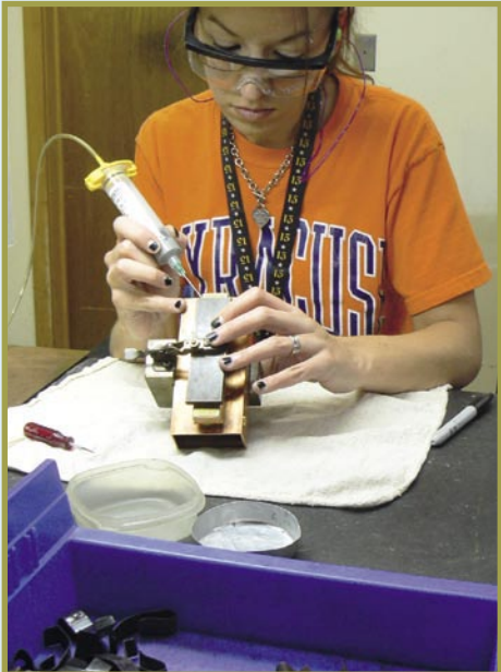
■ Here a filter is mechanically assembled. MFC employee Melissa Bench prepares a filter for the soldering oven...
