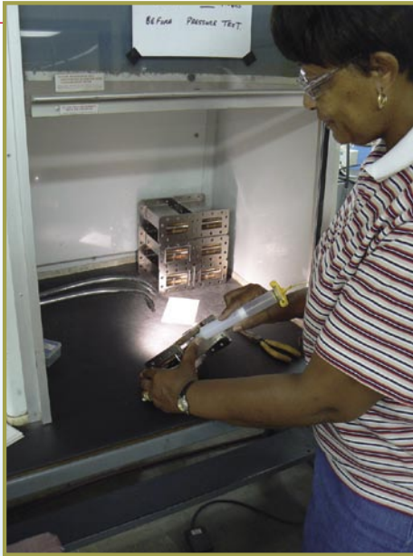
■ The reception probe in the filter is put in place by Vertell Brantley. The glue that is used needs to set for three hours; the filters are stored in this chamber protected from the surrounding air. Thereafter, the filters are fixed with a weather-tight seal.
