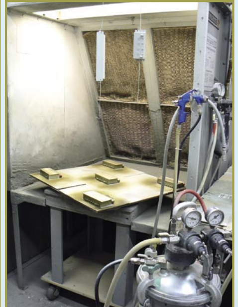
■ MFC virtually does it all by themselves: the completed filters are sprayed here with a protective color coating.
