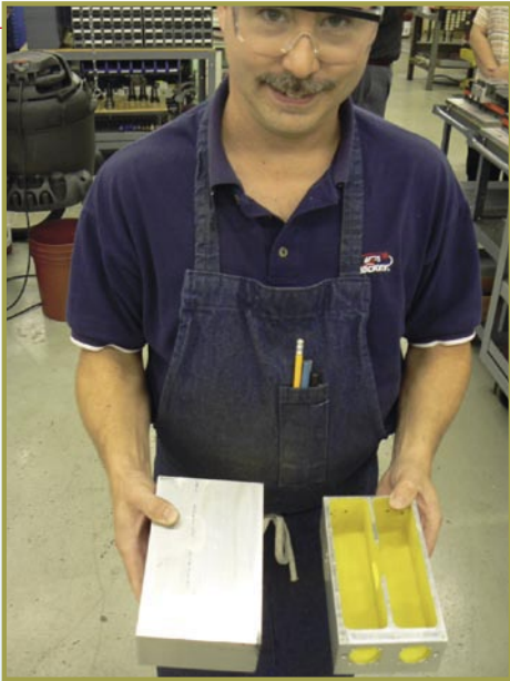
■ Dale Newton shows us the production sequence: out of a solid block of aluminum (left) a complete filter body is milled with all the openings for connectors and screws (right).
