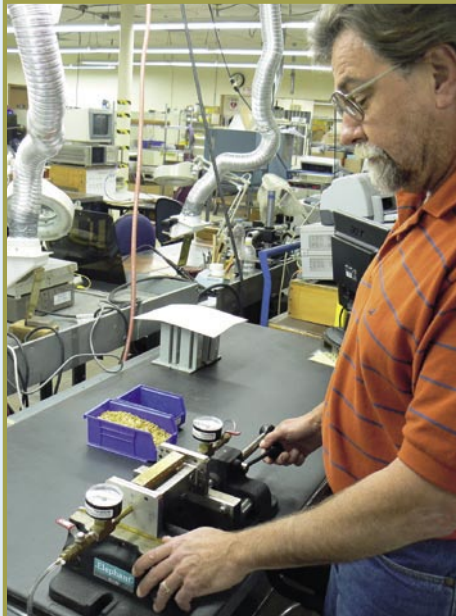
■ Bill Adamo is Quality Control Group Leader and shows us how the weather-tight seal of a filter is pressure tested: "The filter is placed here and pressurized with air at 5 PSI." In this way they can check if the inside of the connector, as well as its mounting to the housing are air tight. "The smallest leak can let moisture in over time and could alter the characteristics of the filter", says Bill Adamo, "We test 100% of our filters!" Every customer can be sure that each and every MFC filter lives up to its high-quality specifications.
