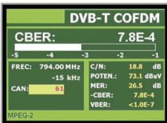
Shows all measurements simultaneously
