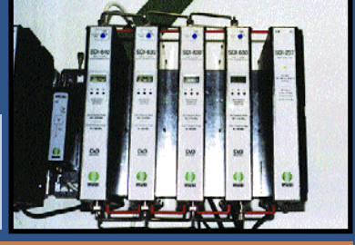
Ikusi, ES-San Sebastian: SDI-630, SDI-640 digital headend, transparent digital transmodulation Info Page: www.satellite-shop.com/Ikusi-SDI630
