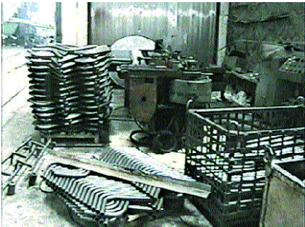
The machine that bends the pipes for the mount
