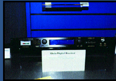
Standard Communication, UK-Watford-Herts: Altea digital receiver a 3rd generation DVB/MPEG-2, supports 4.2.2, 4.2.0, QPSK and 8PSK formats Info Page: www.satellite-shop.com/Standard-altea
