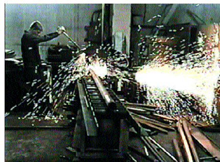
Cutting the pipes to be used in mounts
