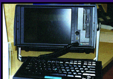
Wandel & Goltermann, FR-Plaisir: WG DTS-A/G system with monitoring, analysis and capture of MPEG-2/DVB transport streams www.satellite-shop.com/WandelGoltermann-WG-DTS
