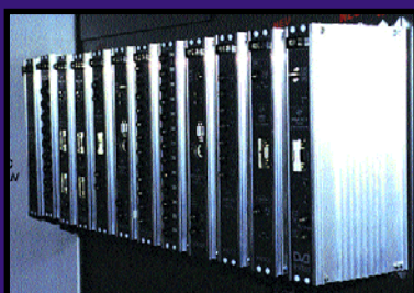
Antech, IT-S. Giovanni La Punta (Catania): Upconverter unit - 13.75 / 14.5 - 17.3 / 18.4 GHz www.satellite-shop.com/Antech-upconverter
