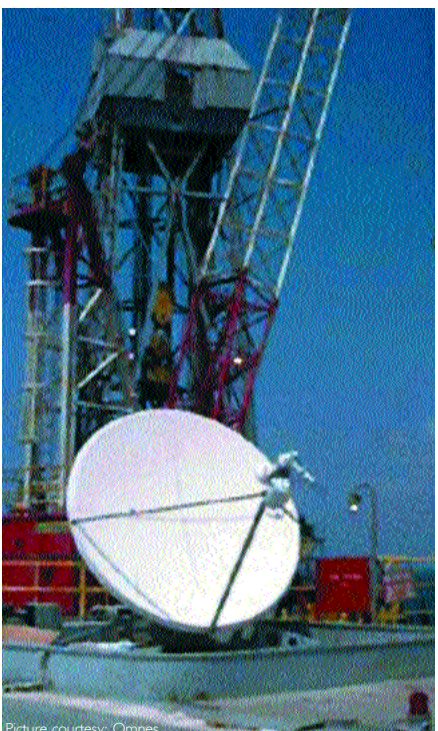
Picture courtesy: Omnes V-Sat antenna on a petroleum platform.
