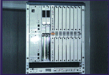
ADC, USA DV-6000 digital video optical transmission system, 16-80 channels high quality over single fibre, distance more than 100 km without translation www.satellite-shop.com/CTV-ADC-DV6000
