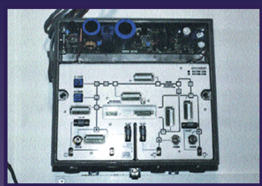
ADC, USA DV-6000 digital video optical transmission system, 16-80 channels high quality over single fibre, distance more than 100 km without translation www.satellite-shop.com/CTV-ADC-DV6000
