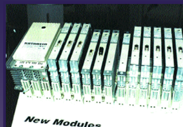
Ircos, Spain Quasar TM 100 TDT for SMATV, selects one input channel in the satellite IF range and converts it to 64 QAM and into the VHF frequency range www.satellite-shop.com/CTV-Ircos-TM100
